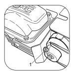
Disconnect the spark plug lead.
